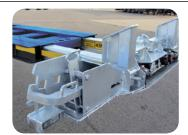
Option: Extension Front front load container 45' and swap within the legal maximum allowed (without special permit to transport). Neck height of 150 mm. Sliding extension guided by bearings and Teflon plates. Galvanized complete set extension to ensure their conservation.
