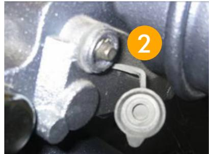
When turning the screw that is in the inside, we will hear an initial “click”. We will release the screw until the brake pads are totally separated from discs.
